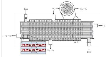
Priming volume minimization by microspheres in the blood compartment (a) and certain fiber configuration of the gas compartment (b) of the novel fiber membrane oxygenator. (source: PCT/EP2022/080548, modified)
